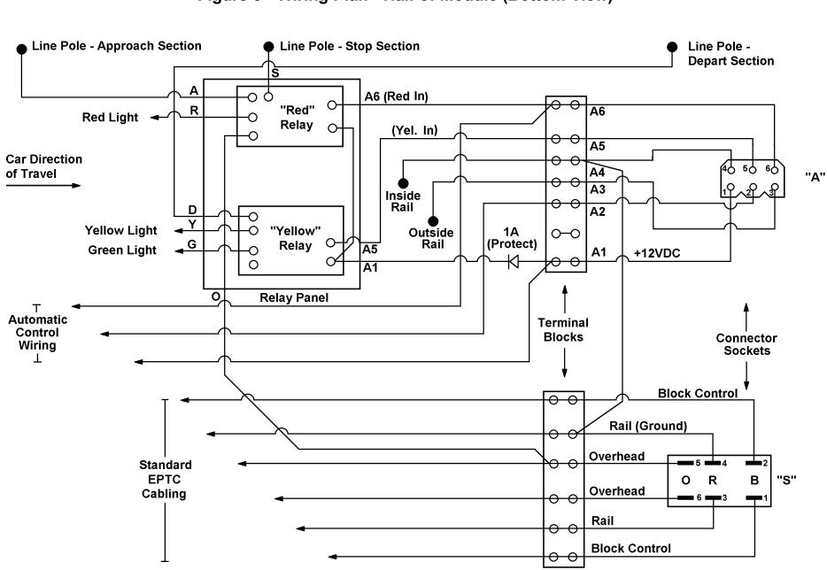
East Penn Traction Club Figure 5 - Wiring Plan - Half of Module (Bottom View)
